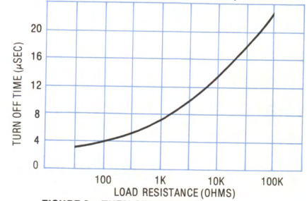
FIGURE 6 - TURN OFF TIME VS. LOAD RESISTANCE (TYPICAL)
